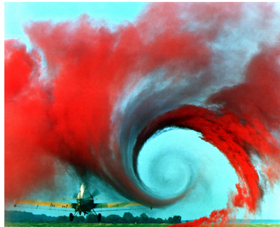
Vortex created by the passage of an aircraft wing, revealed by coloured smoke.
