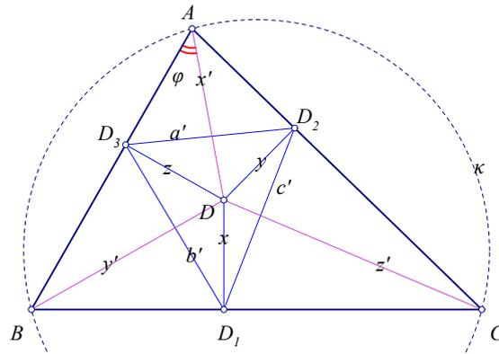
Figure 33: Trilinear relations of the pedal  $D_1D_2D_3$  of  $D$  relative to  $\triangle ABC$
