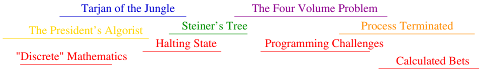
Figure 1.5: An instance of the non-overlapping movie scheduling problem. The four red titles define an optimal solution.
