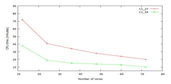
**Fig. 3** Performance of WRF for C1 configuration. CPU time, required for one hour simulation, was recorded. C1\_27 refers to C1 configuration with 27 sec domain d01 timestep and C1\_54 refers to C1 configuration with 54 sec domain d01 timestep. The CPU-time ratio between the two different cases is approximately 2 (it varies between 1.84 and 2.26).
