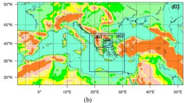
**Fig.2** The two different nested domain configurations (a) 3-domain configuration C1, with horizontal grid resolutions d01: 27 km, d02: 9 km, d03: 3 km, (b) 4-domain configuration C2, with horizontal grid resolutions d01: 27 km, d02: 9 km, d03: 3 km, d04: 1 km.
