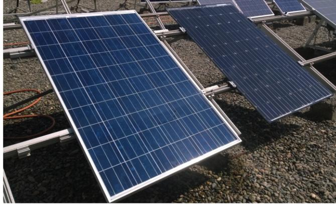
**Figure 2:** Installed PV modules at 25 degrees tilt. On the left is the location of the monofacial polycrystalline module, while on the right is the bifacial one.
