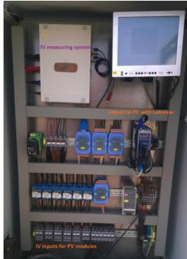
**Figure 3:** IV tracer system with multiple inputs for measuring the output of the monofacial and bifacial modules.**Table 2:** IV tracer system technical specifications
