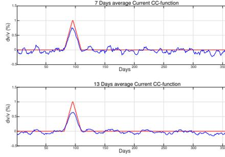
**Figure A1.** In the top plot  $N_{ccc} = 7$  days are used in computation of the reference CC while  $N_{ccc} = 13$  days are used in the bottom plot. In red is the true velocity variation and in blue the estimated one. Using  $N_{ccc} = 7$  days gives a more precise estimation for the maximal value of  $dv/v$  while with  $N_{ccc} = 13$  days the fluctuations around zero are decreased.
