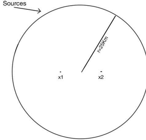
**Figure 1.** Location of the noise sources on a circle,  $\mathcal{C}$ , of radius 25Km and the two receivers at  $\mathbf{x}_1$  and  $\mathbf{x}_2$ . The distance between the two receivers is 10Km.
