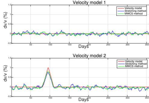
**Figure 3.** Relative velocity change estimation using SM (blue) and MWCS (green) for the constant (top) and the variable (bottom) velocity models of Figure 2.
