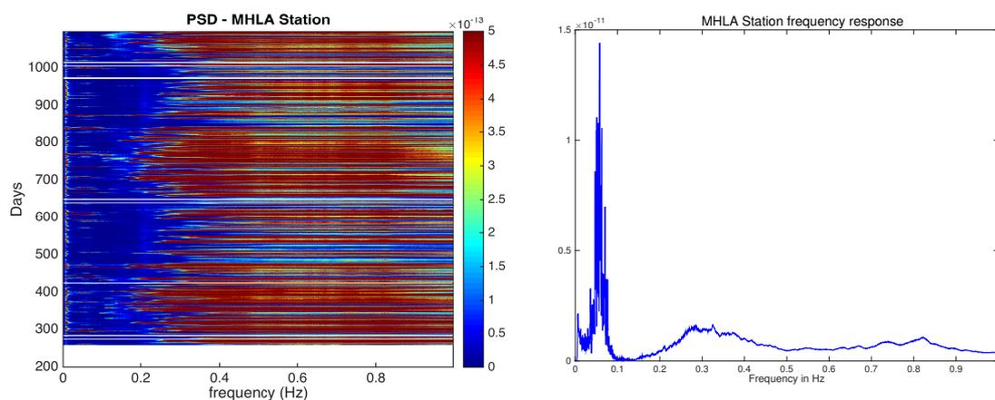
**Figure 12.** Left: The Power Spectrum Density of the station MHLA at Milos. Right: The frequency response of the MHLA station calculated by averaging the daily frequency response of all available days.
