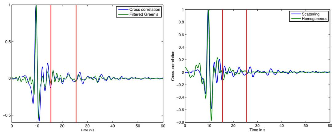
**Figure 8.** Left: The reference CC in the scattering medium compared with the Green's function between the two receivers filtered by the power spectral density of the noise sources. Amplitudes are normalized. Right: The reference CC in the homogeneous and the scattering medium. In both plots, the two red vertical lines indicate the window  $[15.5 - 25.5]$ s.
