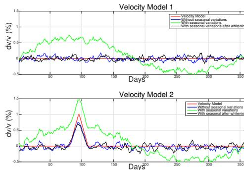
**Figure 5.** Comparison between the estimation obtained for the model without seasonal variations in blue (equation (A.2)), the model with uniform seasonal variations in green (equation (A.5)) and the effect of spectral whitening to the estimation in black for both velocity models. All estimations here are produced using the stretching method.
