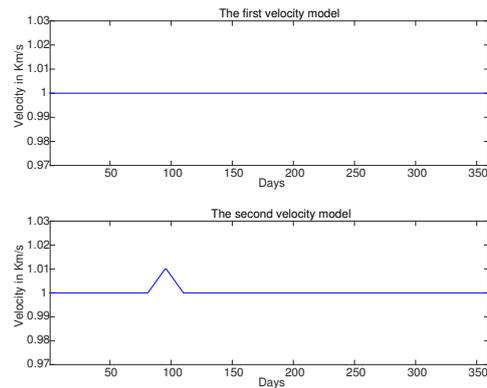
**Figure 2.** The two velocity models. In the top plot the velocity does not change with time and is equal to 1Km/s. In the bottom plot the velocity increases linearly between days 80 and 95 to reach the value of 1.01Km/s and then decreases linearly with the same rate to reach its original value of 1Km/s at day 110.
