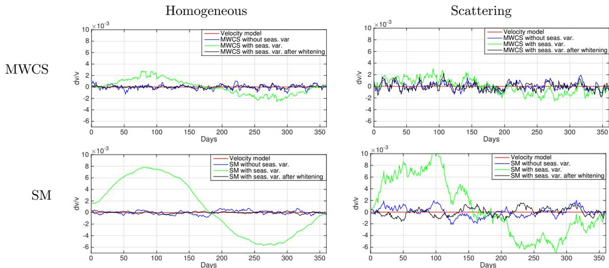
**Figure 10.** Removing the seasonal variations using spectral whitening. The noise sources have anisotropic spatio-temporal fluctuations as described by (A.7)-(A.8). For the SM method, the measurements in the homogeneous medium are performed using the  $[10.5 - 20.5]$ s window while in the scattering medium the  $[15.5 - 25.5]$ s window is used.
