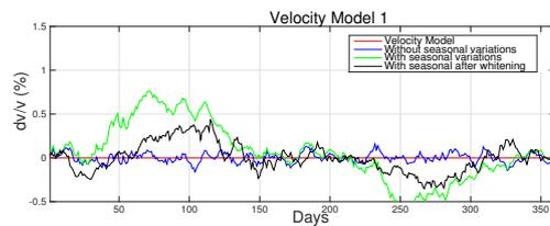
**Figure 6.** The estimation produced by the stretching method for the numerical model without seasonal variations in blue (equation (A.2)), the model of uniform seasonal variations in green (equation (A.9)) and the effect of spectral whitening to the estimation in black.
