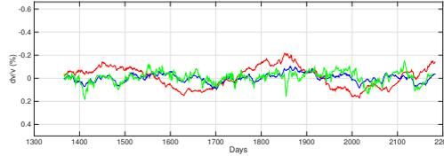
**Figure 13.** The estimation between the pair MHLO-MHLA located on the island of Milos when we use spectral whitening (blue) and when we do not use it (red). Here  $N_{ccc} = 21$  Days. We also plot with green the estimation of the MWCS method which is not affected by the seasonal variations.
