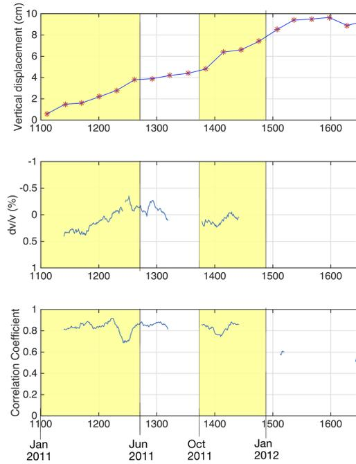
**Figure 16.** Top: Accumulated elevation of the GPS station NOMI in Santorini (Saltogianni et al., 2014 ). Middle: The estimation of  $dv/v$  using the stretching method. Bottom: The correlation coefficient of the stretching method.
