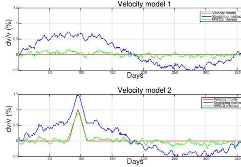
**Figure 4.** Relative velocity change for the first (top) and the second (bottom) velocity model using SM (blue) and MWCS (green) for the velocity models of Figure 2. Only the stretching method is affected by the seasonal variations since those are uniform with respect to the locations of the noise sources.
