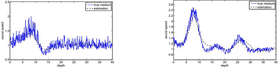
FIG. 3.8. *Velocity estimation in the case of stronger variation of the background speed  $c(z)$ . We show with the blue solid line the true speed  $v(z)$  and with the black dotted line the estimated  $c(z)$ . The abscissa is negative depth scaled by  $\lambda_o$  and the speed is in units of km/s.*
