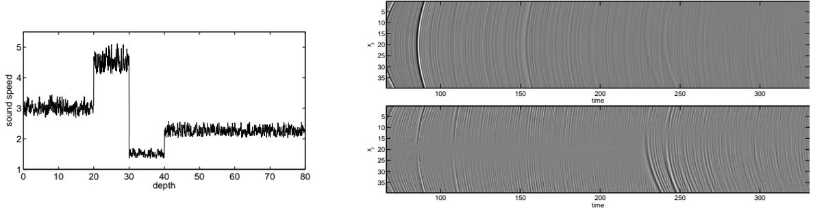
FIG. 3.2. Left: Sound speed  $v(z)$  in  $\text{km/s}$  vs. depth in hundreds of meters. Right: Traces before (top) and after (bottom) annihilation. The abscissa is time scaled by the pulse width of  $0.02\text{s}$ . The ordinate is the receiver location in hundreds of meters. The source is at the center of the array and the array is linear of aperture  $a = 4\text{km}$ .
