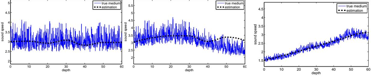
FIG. 3.7. *Velocity estimation results. We show with the blue solid line the true speed  $v(z)$  and with the black dotted line the estimated  $c(z)$ . The abscissa is negative depth scaled by  $\lambda_o$  and the speed is in units of km/s.*
