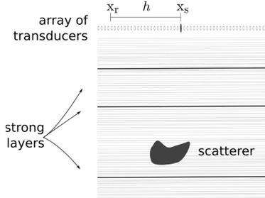
FIG. 2.1. Schematic of the imaging setup. A compactly supported scatterer is buried in a finely layered medium. The array of transducers lies on the top  $z = 0$  and it consists of a source at location  $\vec{\mathbf{x}}_s = (\mathbf{x}_s, 0)$  and receivers at points  $\vec{\mathbf{x}}_r = (\mathbf{x}_r, 0)$ . The medium is finely layered and it may also have some strong scattering interfaces, which we draw with thick black lines.
