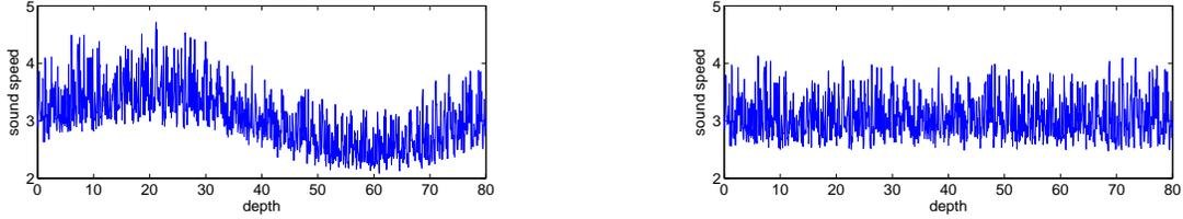
FIG. 3.1. Sound speeds  $v(z)$  considered in the numerical simulations. We take three different strengths of the fine scale fluctuations: 13%, 30% and 50%. The plots are for 30% fluctuations. The depth  $z$  is in units of  $\lambda_o = 100\text{m}$  and the speed is in units of  $\text{km/s}$ .
